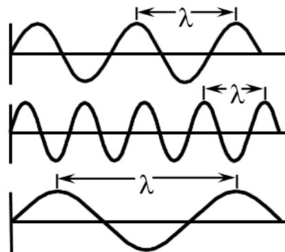
The relationship between frequency and wavelength can be demonstrated using a slinky simulating transverse waves. If a person moves the slinky up and down faster, the frequency increases. However, the distance between the peaks of the slinky wave (wavelength) becomes shorter.
