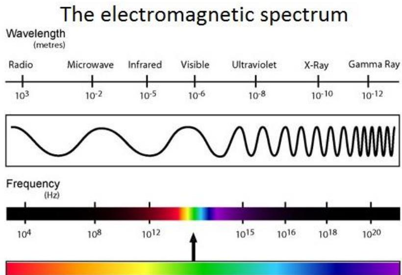
The electromagnetic spectrum is the range of various electromagnetic waves of different frequencies and wavelengths. These waves have many different properties. However, as electromagnetic waves are self-propagating, they do not require a medium to travel.
